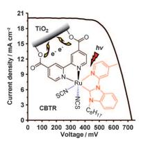
A new generation: The incorporation of N-heterocyclic carbene/pyridine-based ruthenium sensitizers derived from benzimidazolium salts into dye-sensitized solar cells results in superior current densities, cell voltages, and photoelectric conversion efficiencies. The performance of a solar cell sensitized with CBTR (see picture) exceeded that of the traditional N719 cell.
